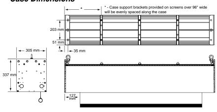
\*Please Note: Optional wall brackets add 1¾" per bracket to case length. Wall mounting bracket hole location is 1" from end of case.
