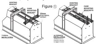
With typical installation, brackets may be angled to meet installation requirements. Please Note: A Hoisting Bracket is included on each end of the case to aid in overhead installation of the Ultimate Access XL case.
